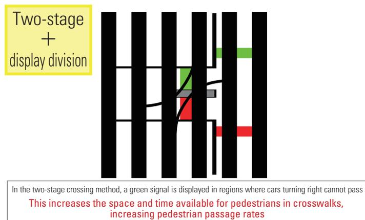
Figure 2. Two-stage crossings and signal display division
