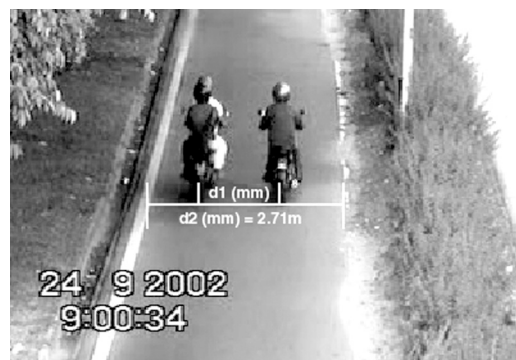
Fig. 1 Distances between centers of rear tires (d1) and effective width (d2) as the faster motorcyclist passed the slower ones
