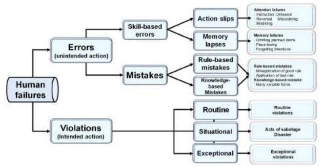
Figure 2-14 Types of human failures / errors Source: SRK Framework, Rasmussen, 198; Introduction to Health and Safety at Work, 2007, 3rd Edition
