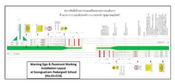
Figure 8-7 The increase of various safety equipment warning the driver to reduce speed
