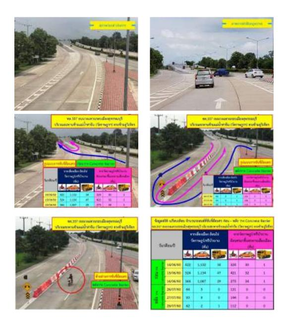
Figure 8-30 Physical features and driving in violation of traffic rules, including statistics on the number of cars in violation of traffic rules, comparing before/after concrete barrier and directing the driver in the designated traffic lane.
