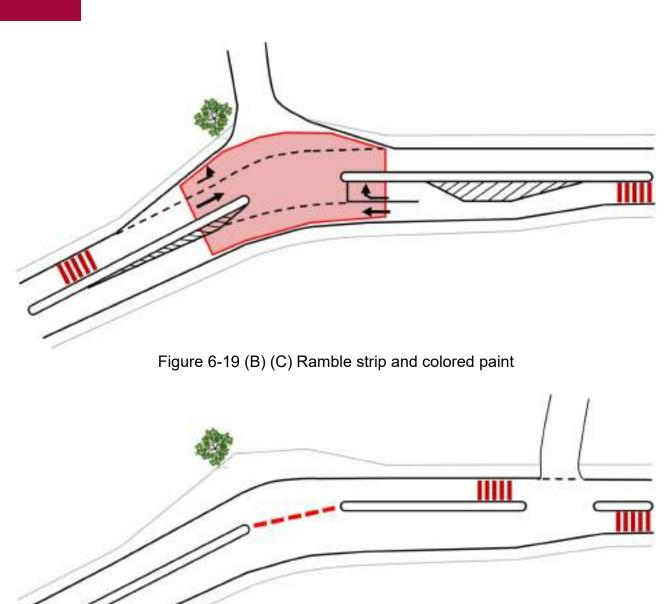
Figure 6-20 (D) Shifting the connection position of the local road
