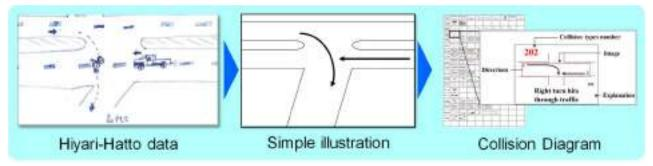
Figure 5-4 Process to identify collision type
