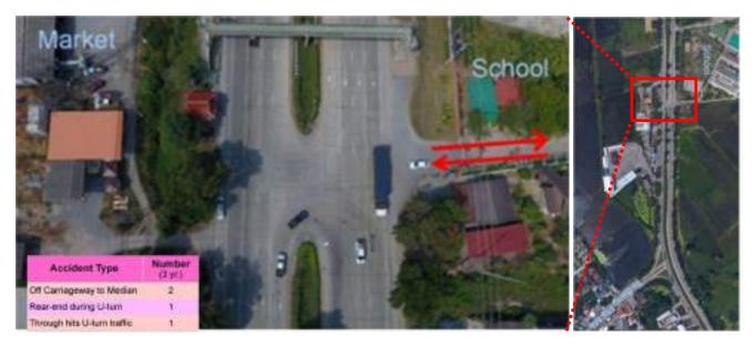
Figure 8-6 Physical characteristics of the road section from 61+250 km to 61+600 km in front of Soongsumarn Padungwit School
