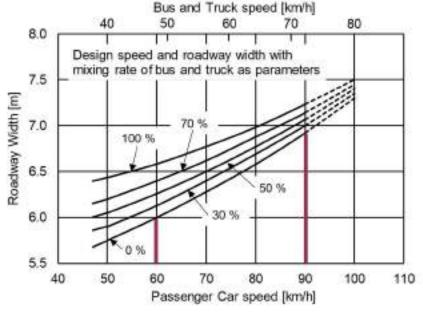
Figure 1-7 Relationship between vehicle speed on two-lane road and roadway width
