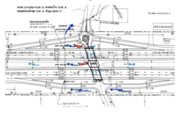
Figure 8-19 (Cont.) The construction plan and traffic patterns, including drainage, at the Po Koi intersection area
