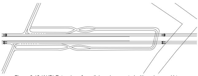
Figure 6-12 (A)(B) Extension of parallel road connected with underpass U-turn
