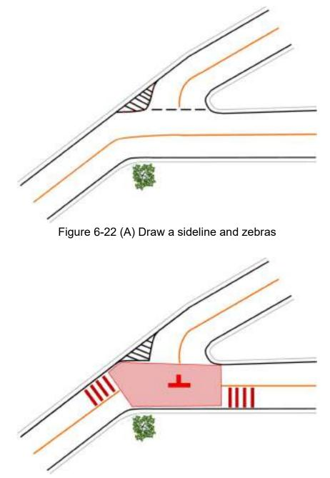
Figure 6-23 (B) T-shape with colored pavement, center making, and rumble strip
