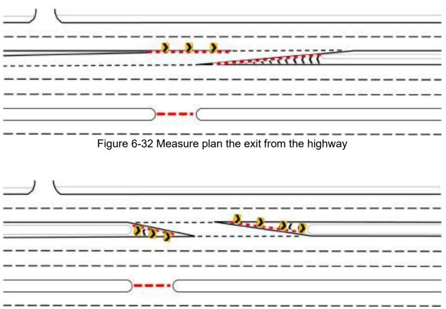
Figure 6-33 Measure plan at the entrance from the parallel roads
