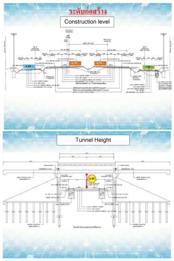
Figure 8-18 (Cont.) The construction plan and traffic patterns, including drainage, at the Po Koi intersection area
