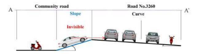
Figure 6-16 Cross section of curve section (existing condition) invisible
