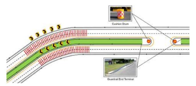
Figure 6-35 (A) (B) Rumble strip and guardrail, cushion drum
