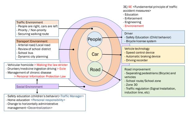
Figure 1-1 Schematic diagram of traffic accident countermeasures on school route
