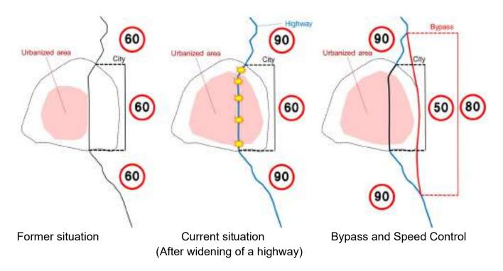
Figure 6-38 Fundamental idea of speed control by wide area
