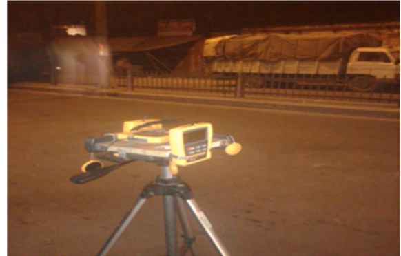
Figure 5. Assembly of 3 light meters mounted on a tripod.
