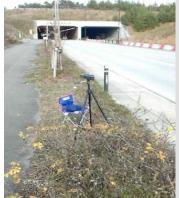
Upstream camera (showing dummy radar gun)
