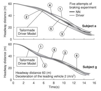
Fig. 7 Change in the headway distance between NN and the driver
