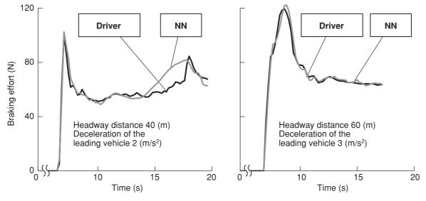
Fig. 2 Simulation of the driver's braking (Subject a)
