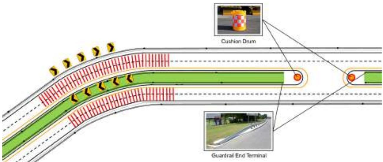
Figure 6-35 (A) (B) Rumble strip and guardrail, cushion drum
