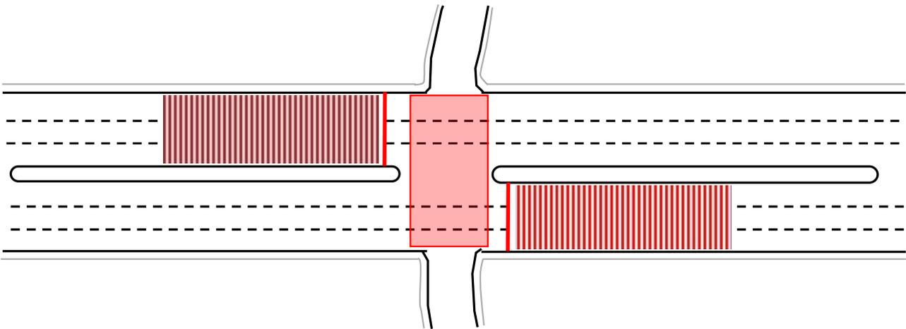
Figure 6-2 (A) Rumble strips and road markings
