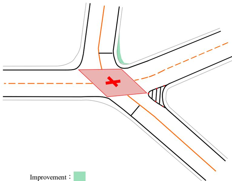
Figure 6-28 (B) T-shape with colored pavement, center making, and rumble strip
