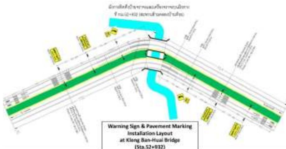
Figure 8-2 Installment plan of safety equipment
