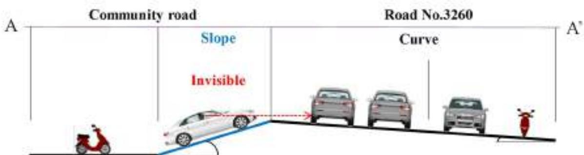
Figure 6-16 Cross section of curve section (existing condition) invisible
