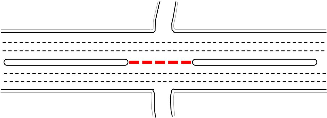
Figure 6-4 (C) Closing U-turn section
