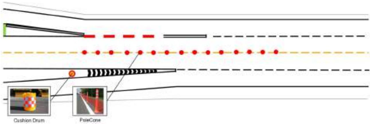
Figure6-8 (A) Installing the Pole Cone on median and (D) the cushion drum to the separator
