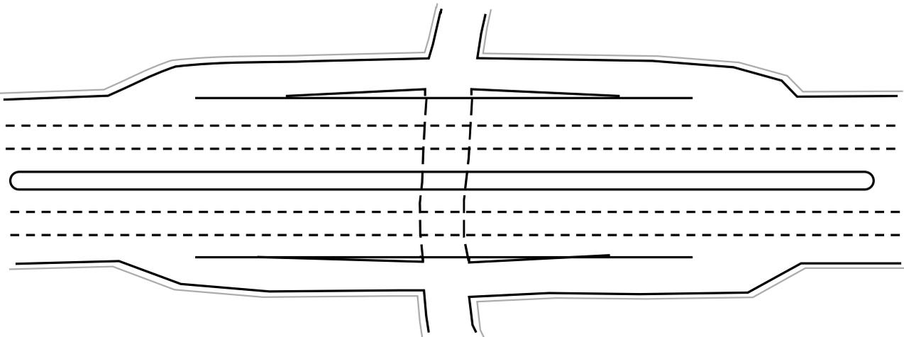
Figure 6-5 (D) Setting up a frontage road paralleled with a highway and closing U-turn section
