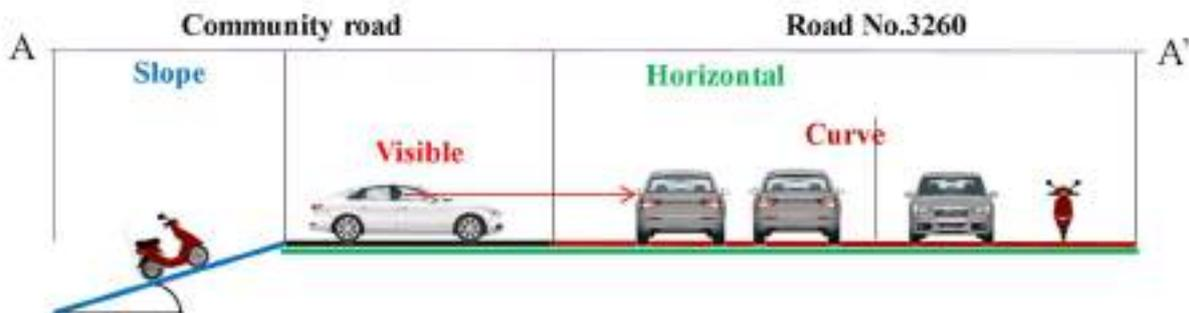
Figure 6-18 (A) Proposed cross section
