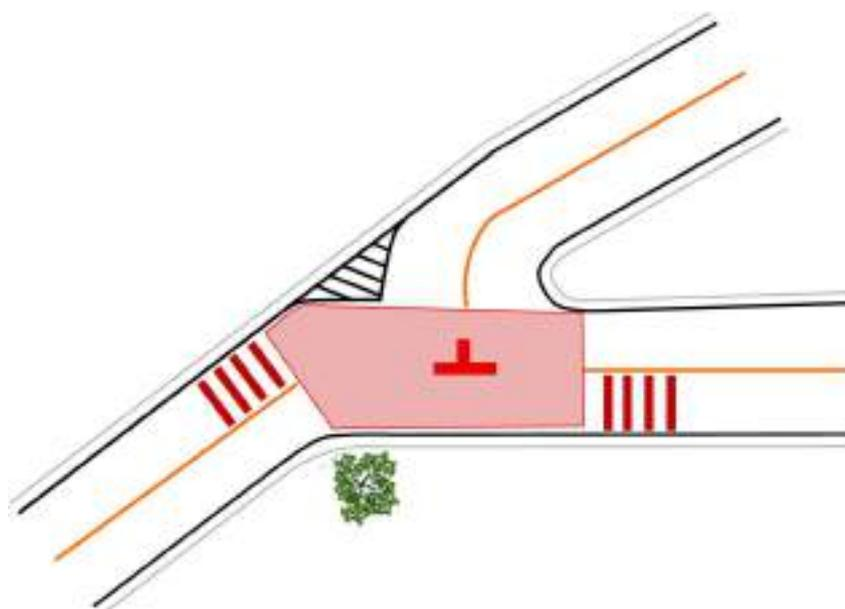
Figure 6-23 (B) T-shape with colored pavement, center making, and rumble strip
