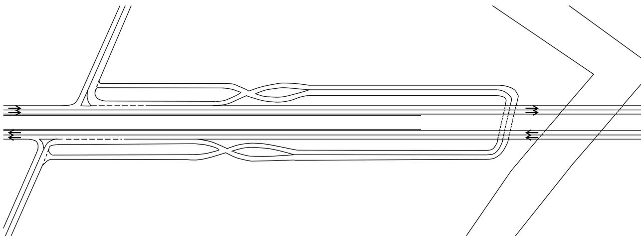
Figure 6-12 (A)(B) Extension of parallel road connected with underpass U-turn
