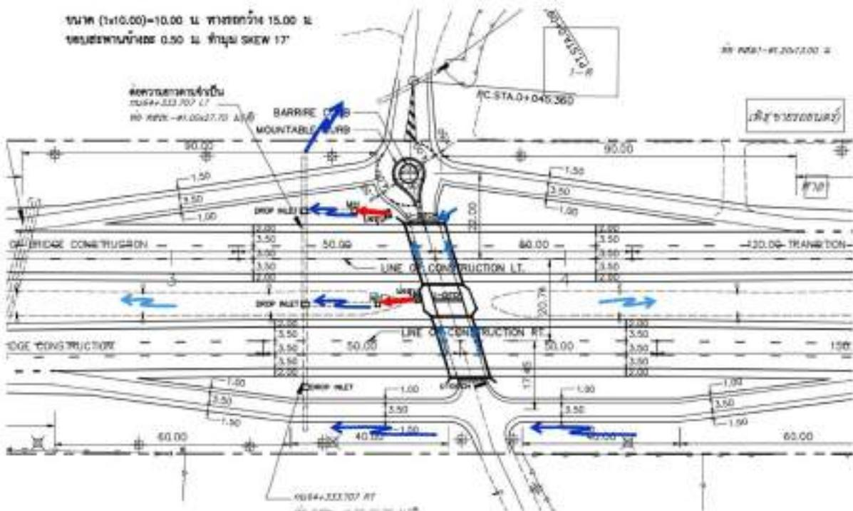
Figure 8-19 (Cont.) The construction plan and traffic patterns, including drainage, at the Po Koi intersection area
