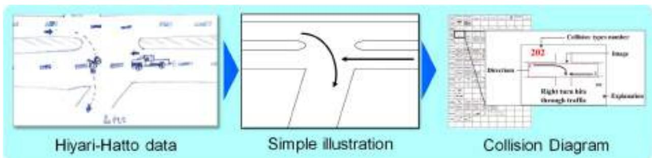
Figure 5-4 Process to identify collision type
