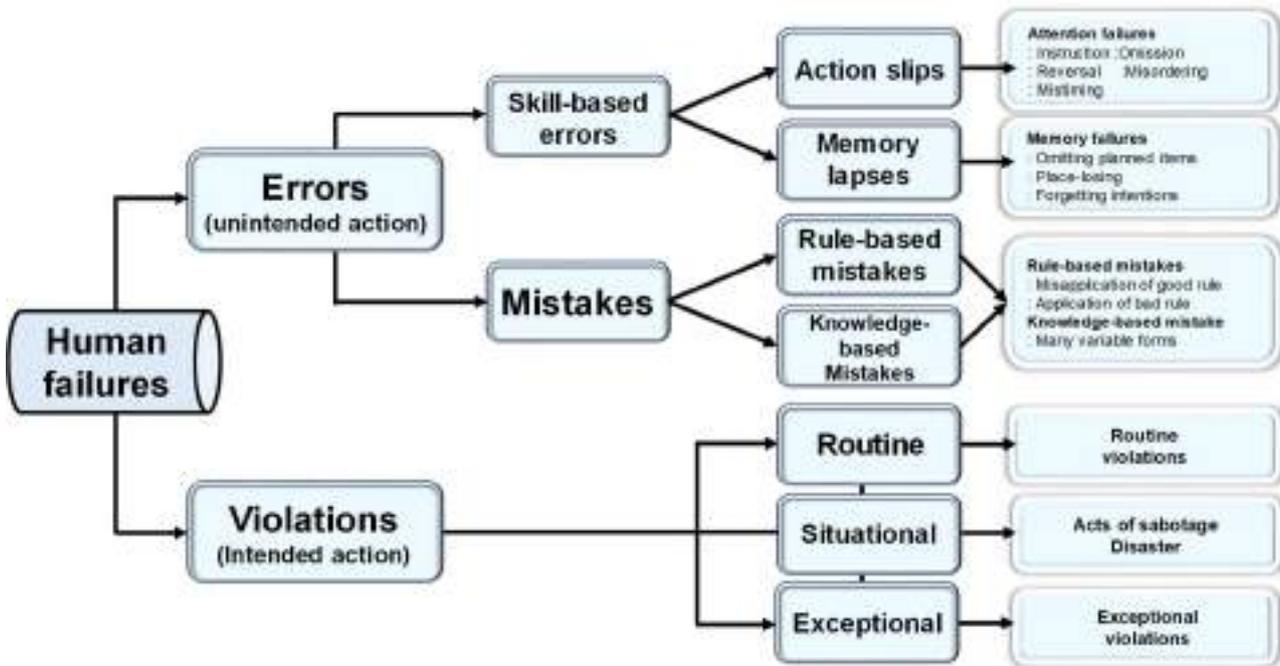
Figure 2-14 Types of human failures / errors
