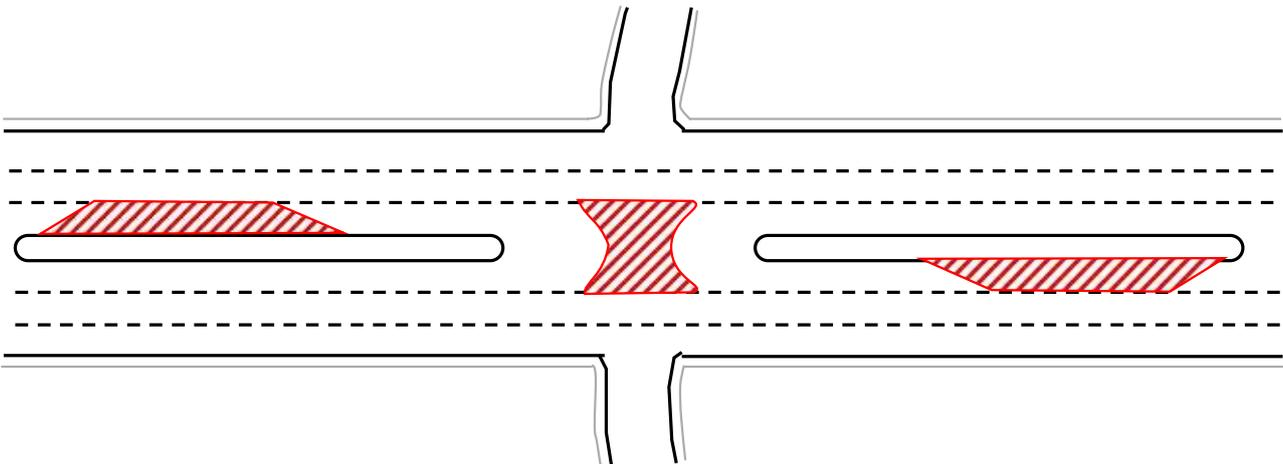
Figure 6-3 (B) Setting up U-turn lane and road marking
