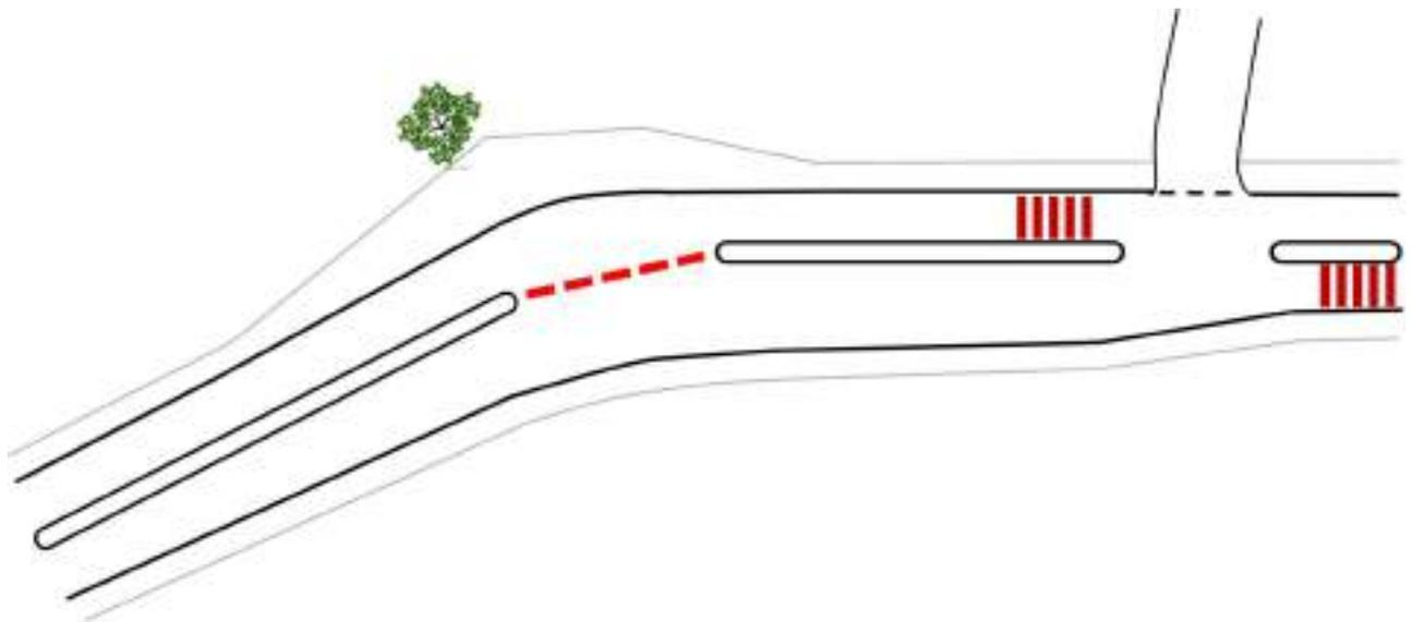
Figure 6-20 (D) Shifting the connection position of the local road
