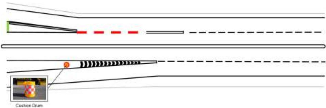
Figure 6-9 (B) Installing the median strip
