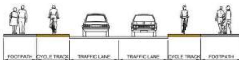
Figure 1-4 Cross section of separation of road, bicycle lane, and sidewalk
