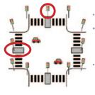
A central island is established in the crossing A pedestrian crossing signal is added to the central island
