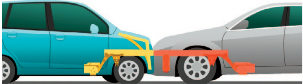
Figure 3. Schematic diagram of crash-compatible car bodies 2)
