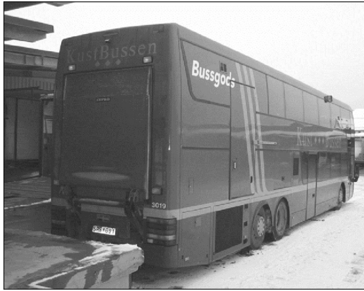
Fig. 6 A typical double-decked, subsidized, wind sensitive, coach with rear baggage and goods compartment further impairing stability. This type of coach is used for combined transport of passengers and goods in rural areas in Sweden. (Photo: P. Albertsson)
