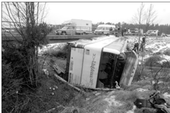
Fig. 5 A major single coach crash with 34 injured caused by severe cross-wind and slippery road conditions 3 (Photo: L. Danielsson)
