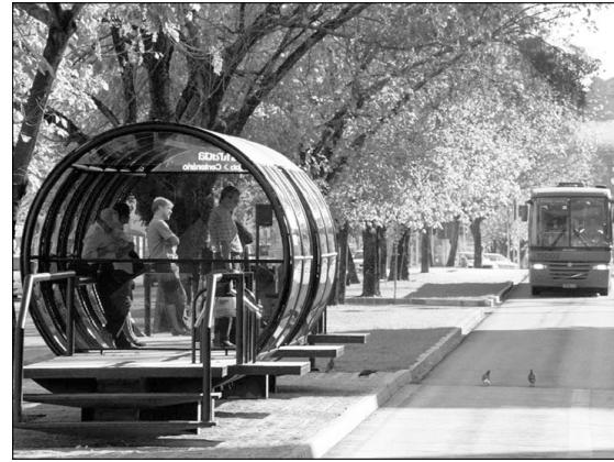
Fig. 7 An example from Curitiba in Brazil of a public transport system, minimizing level problems in boarding and alighting, facilitating and speeding up exchange of passengers and giving shelter to waiting passengers who pay before entering the tube. The system was built in cooperation with the bus manufacturer Volvo.
