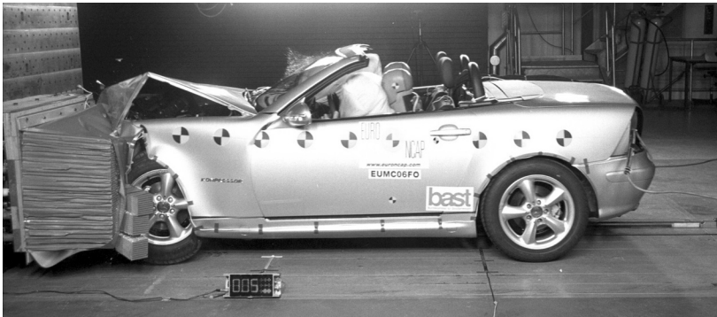
Fig. 4 Crash in the vehicle engineering test facility
