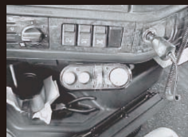
Howard Power Center Steering System
