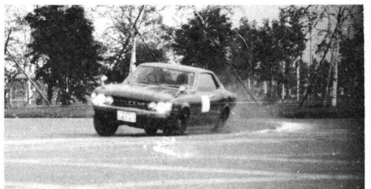
Fig.10 R=40m, V=60km/hの左旋回実験 車体の傾き=7.6° タイヤ=175/70HR13-NT253 Left turning experiment under the condition : R=40m, V=60km/h
