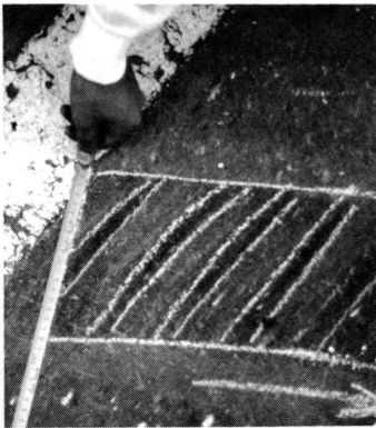
Fig.11-1 左の旋回実験で発生した左前輪タイヤの横すべり痕 Side slip marks of left front tire during left turn spin test
